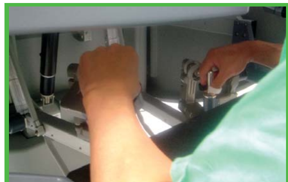
Figure 1. Surgeon operating the two handles in the main console which control the robotic arms of the da Vinci Surgical System
