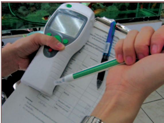
Figure 2: ATP measurement by a hand-held device to provide real-time feedback on effectiveness of cleansing.
