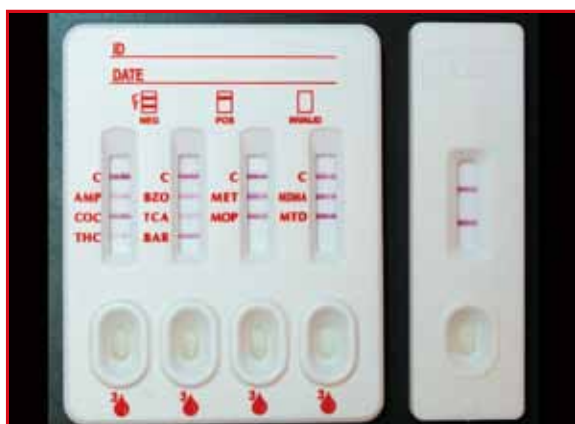
Figure 1: Bedside urine immunoassay kits for screening of abusive substances, from urine specimens produced by the author who had no previous exposure. Both kits showed negative results. Faint lines imply negative results. Left panel, ABON™ Multi-line Screen Test Device. Right panel, ABON™ One Step Drug Screen Test Device for Ketamine.
