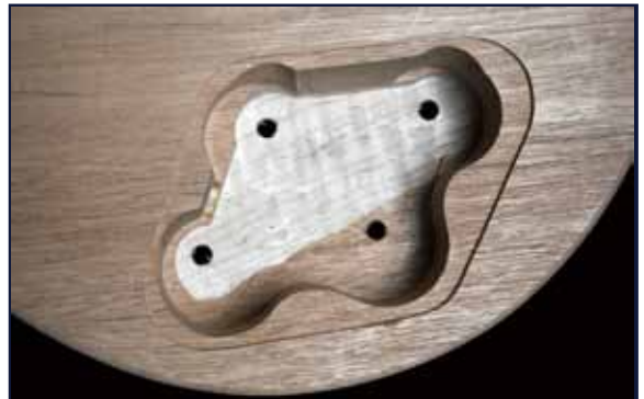
Fig. 11: Secondary Routing performed on control cavity to expose maple, mahogany transition
