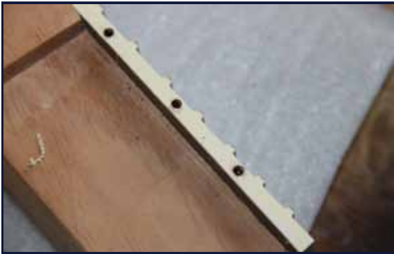
Fig. 17: Tortoise patterned celluloid side dots added after binding glue sets
