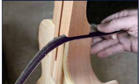
Fig. 20: Sanding of neck joint to insure a flush snug fitting to body.
