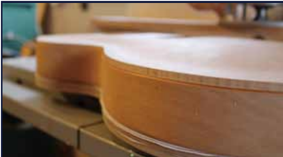
Fig. 8: Channel routed for binding to fit in later, made via a specialized routing bit
