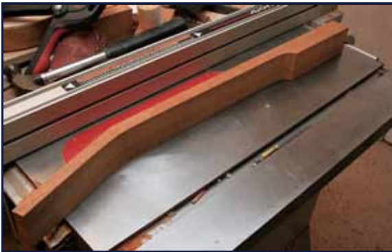
Fig. 18: Neck blank cut into rough shape, and left to rest to prevent wrappage
