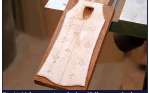
Fig. 21: Mahogany wings glued on. Holly veneer glued headstock with template for later cutting and reference.
