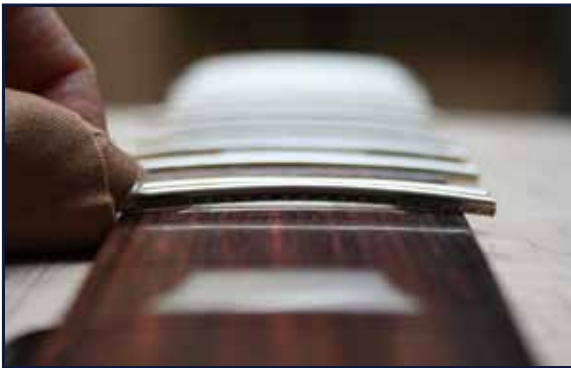
Fig. 15: Fret wire is pre-bent and hammered into the prepared slot; excess ends are nibbed off
