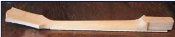
Fig. 24: Final sanding done with sandpaper and steel wool, to ensure smooth neck surface
