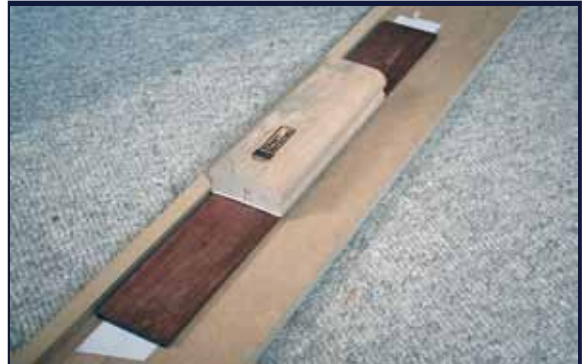
Fig. 12: Radiusing the Brazilian Rosewood fretboard with successive grits of sandpaper
