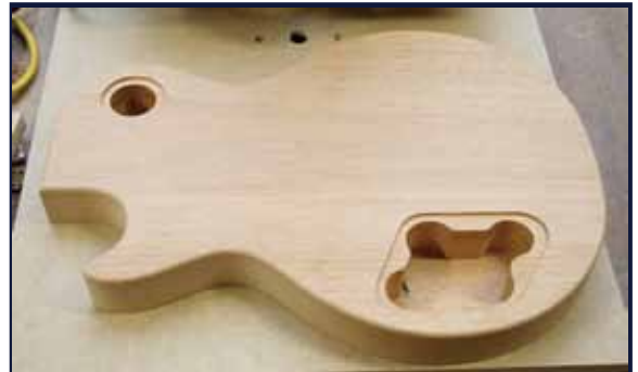
Fig. 4: Control cavity and toggle switch cavity preliminary routing done
