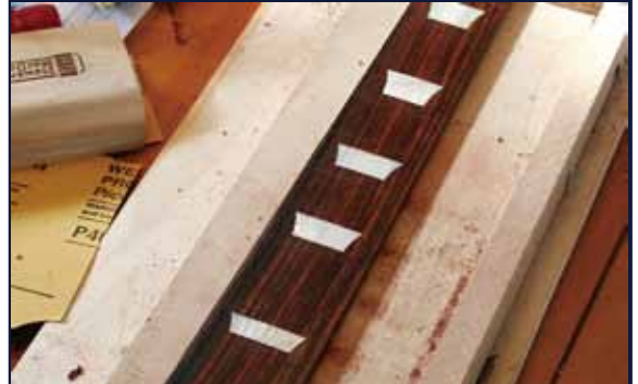
Fig. 14: Inlays are routed from templates and glued with acetate-based glue mixed with saw dust
