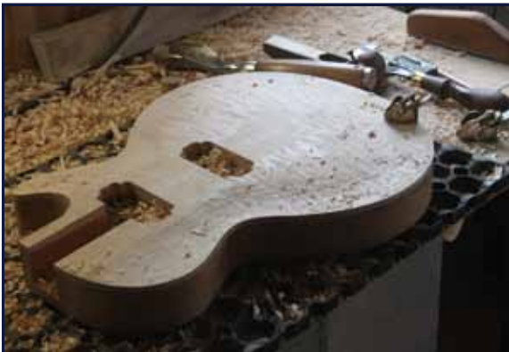
Fig. 7: Shaping of top curve with an assortment of chisels followed by violin planes and scrapers before finally finishing with successive finer grades of sandpaper
