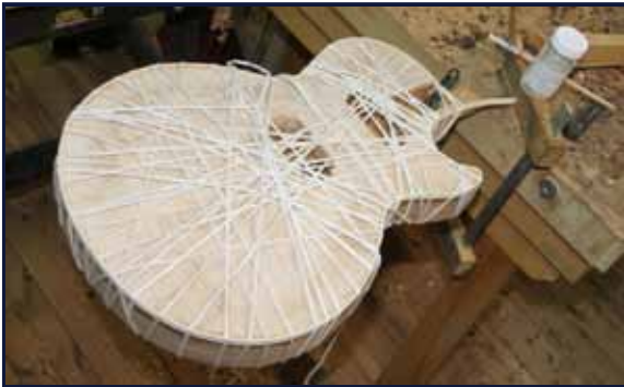
Fig. 9: ABS plastic binding is wrap around the binding channel with heat gun and glued in place with acetone-based glue. A long roll of cotton thread is then wound across to body to insure tight fit of binding while it sets into place.
