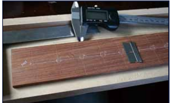
Fig. 13: The fretboard is first trued with a bob plane and then radiused to specification with a sanding block. Fret locations are measured out via the Rule of 18.
