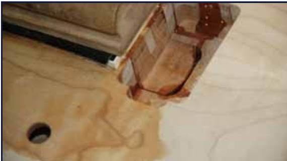
Fig. 25: Body and neck glued together again with hyde glue, excess if wiped off with a damp cloth before letting joint solidify and rest.
