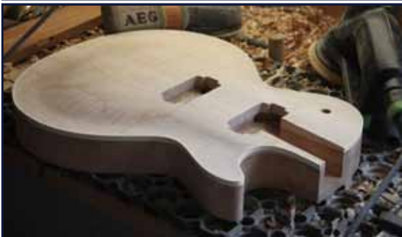
Fig. 10: The binding is scraped with scalpel after which the pickup plane is routed flush to neck angle before final sanding
