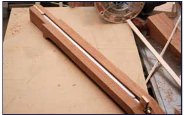
Fig. 19: Neck tenon cut with band saw before finishing with hand chisels. Trial fitting of premade truss rod after channel was routed.
