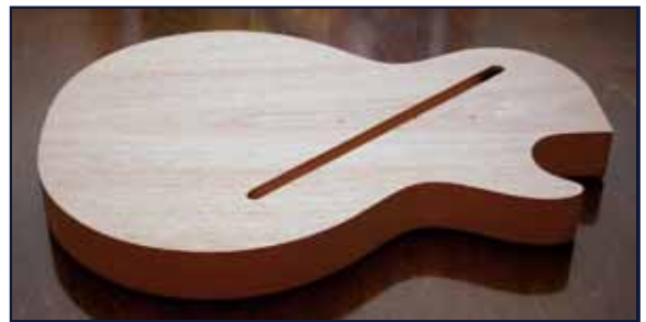
Fig. 3: Body blank is first trued with planer. Rough outline of guitar body is cut with band saw and sanded to size with spindle sander. Toggle switch canal routed
