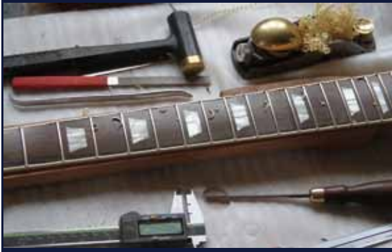
Fig. 16: Royalite binding glued to fingerboard, excess binding scraped with No 15 scalpel, before filing to smoothness. Side dots added after binding glue sets.
