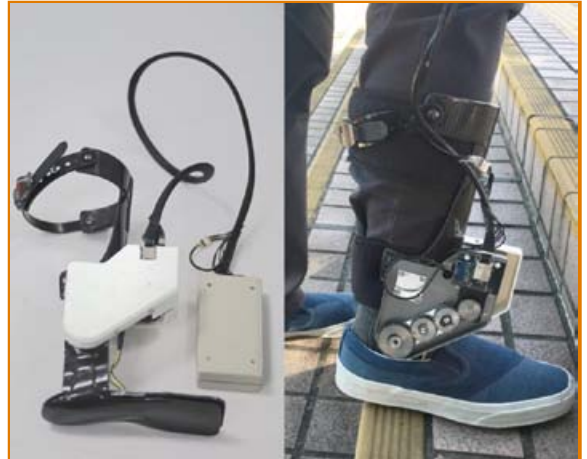
Fig. 1. Exoskeleton Ankle Robot for providing gait assistance of stroke patients in level ground walking and stair ambulation. (Personal collection)
