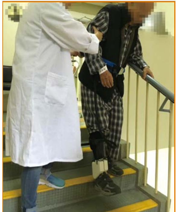
Fig. 2. A stroke patient wearing the Ankle Robot when he is participating in gait training on stairs. (Personal collection)
